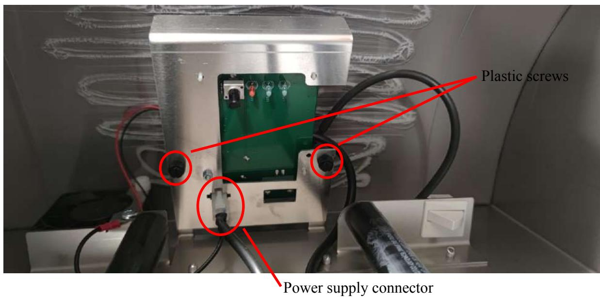
To replace the PCB (Printed Circuit Board), you need to loosen the 2 (plastic) screws that hold the plate with the PCB on top. First unplug the power cable on the lower side (see picture above). Result:
