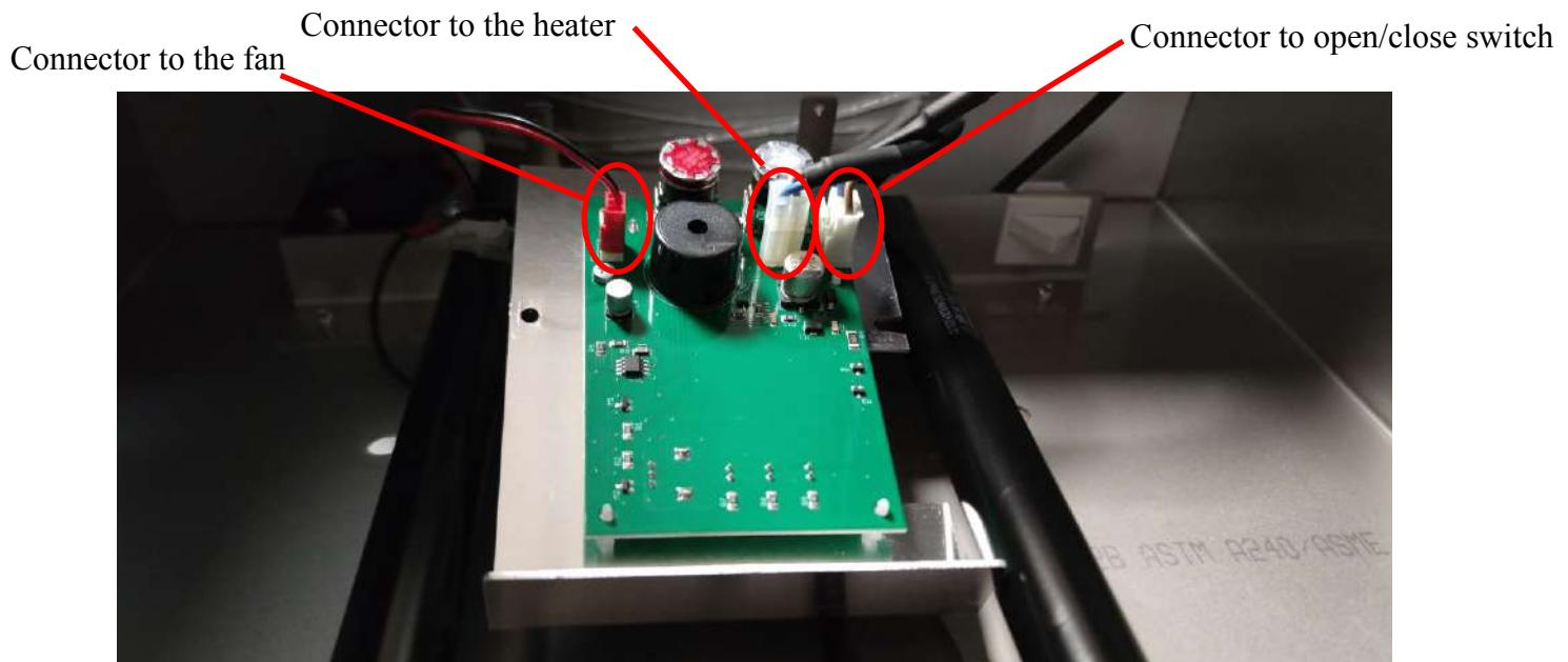
When the plate with the PCB on top is loose, you need to uncouple the electrical remaining connections:
