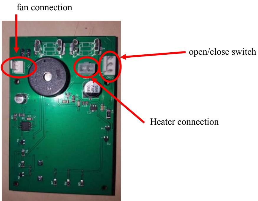
Before attaching the PCB on the drawer using the place holders, please attach the connections as described in the picture above. When these three connections are done, place the PCB on the drawer using the white place holders. The power connection, the LEDS and the turn knob should fit through the drawer plate (some times you need to "squeeze" a little).
