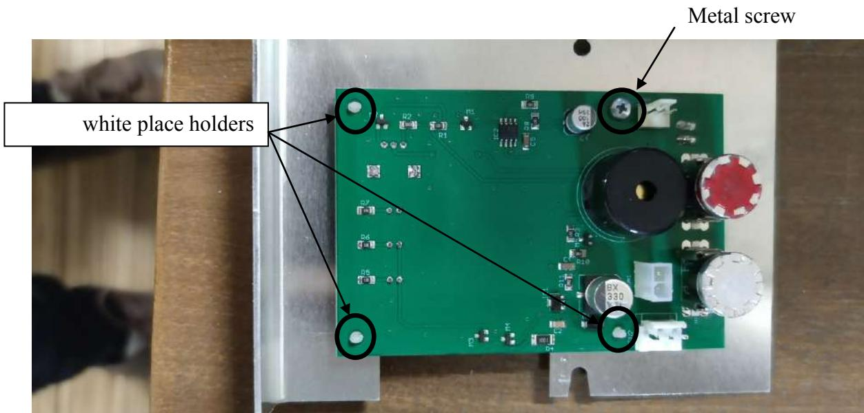
The white place holders can be removed by using a pincer or you nails. When you pinch on the lower side, you can push the white place holders through the hole. Unscrew the screw when applicable.
